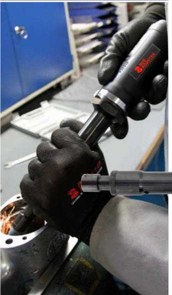
RED ROOSTER die grinders are extremely suitable for deburring applications as well as weld seam finishing and general die grinding applications.
