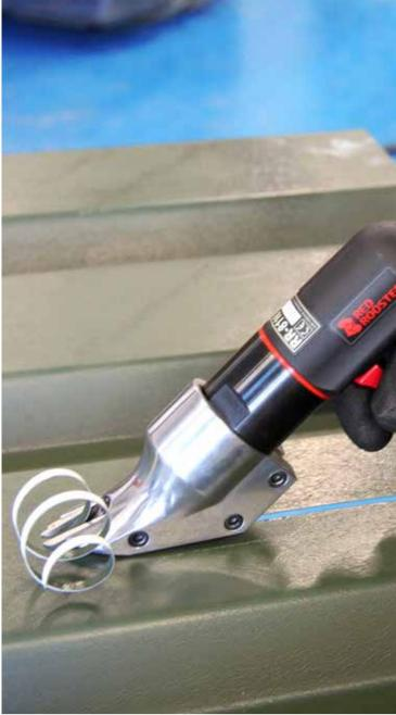
The Red Rooster RR-8110 sheet metal shears remove a narrow strip from the sheet to be cut. Ideal for fast cutting of sheet metal, makes a tight cut without deforming the sheet metal. Also suitable for curved sheet metal such as thin-walled pipes. The head is adjustable 360°.
